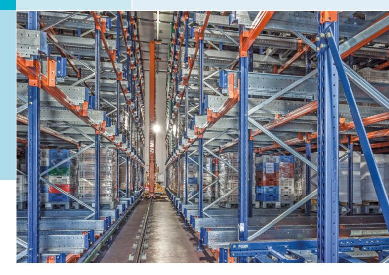
This system involves the incorporation of automated equipment in the handling processes of high-density warehouses. As a result, the forklifts are replaced by stacker cranes or transfer cars carrying the Pallet Shuttle and the load in their cradle.
