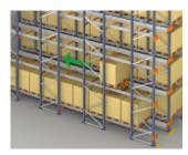
STEP 3 The shuttle raises one pallet slightly and then rolls
