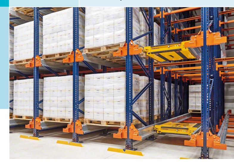
This is a high-density pallet storage system which facilitates the independent loading and unloading of goods from an electric shuttle called a Pallet Shuttle, eliminating the need for forklifts to enter the racking.
