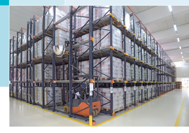
This storage concept consists of a set of racking units which form an internal lane with support rails for the pallets. The forklift enters the lane with the load elevated above the support rail that it will be placed upon.
