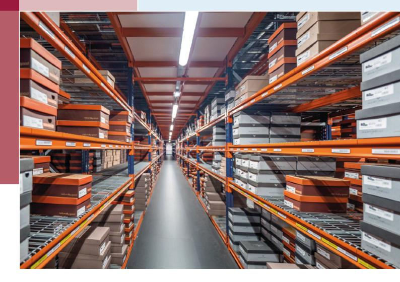
Longspan shelving is designed for warehouses where goods are deposited and removed manually from shelves. This system also makes optimal use of warehouse height, as the higher levels can be accessed mechanically by devices that lift the operator to the required height (stacker cranes or order picking forklifts) or via gangways located between shelves.
