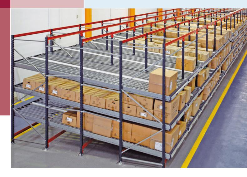
Live storage for picking. Goods are placed onto sloped roller tracks where they then roll at a controlled speed towards the lane exit by the force of gravity.
