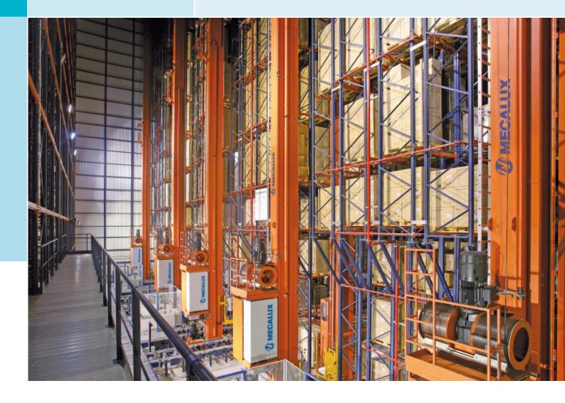
Stacker cranes are machines designed for the automated storage of materials by means of automatic mechanical movements. Materials are inserted and extracted at the same time (known as a combined cycle). This increases the productivity of the installation and also reduces the resources required for it to function.
