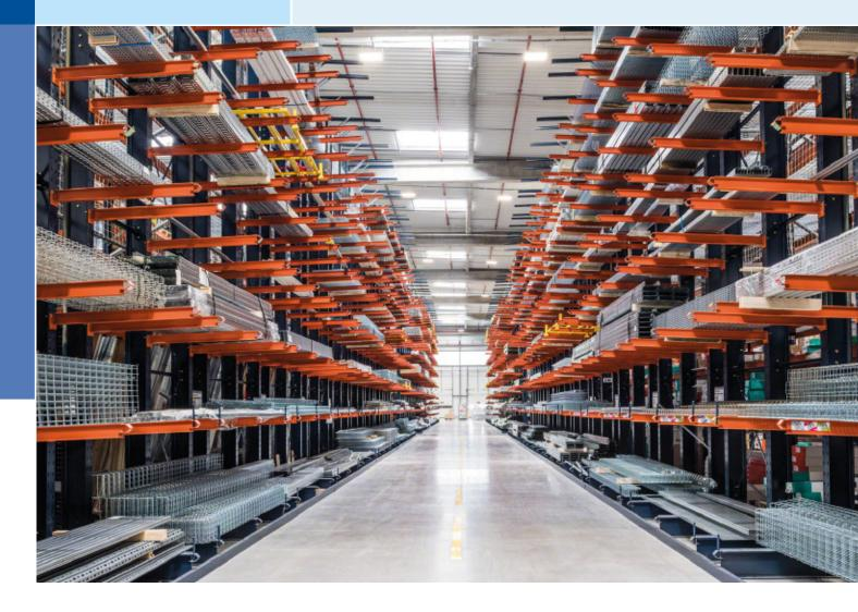
The system consists of columns with a vertical beam and one or two horizontal beams at the base to provide stability. A series of arms are attached, onto which the load is placed.
