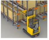
STEP 1 A forklift places a Pallet Shuttle on the level where goods are going to be stored.
