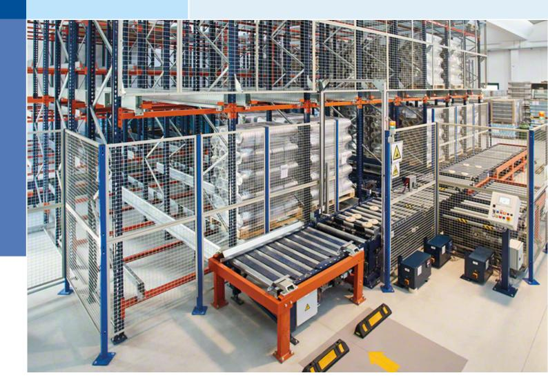
These create a protected space in work areas where there is automated equipment and robotics. They also keep the area free of possible materials shed by the action of machines.
