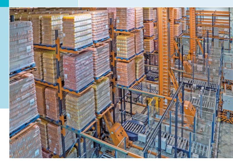
Automatic trilateral stacker cranes make it very easy to automate warehouses with conventional racks where a manually operated lift truck is used, both in pre-existing warehouses and in new facilities.
