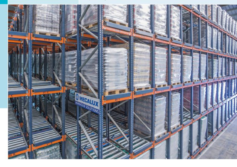
Live storage racking features roller tracks on a sloped lane to allow pallets to slide over them.
