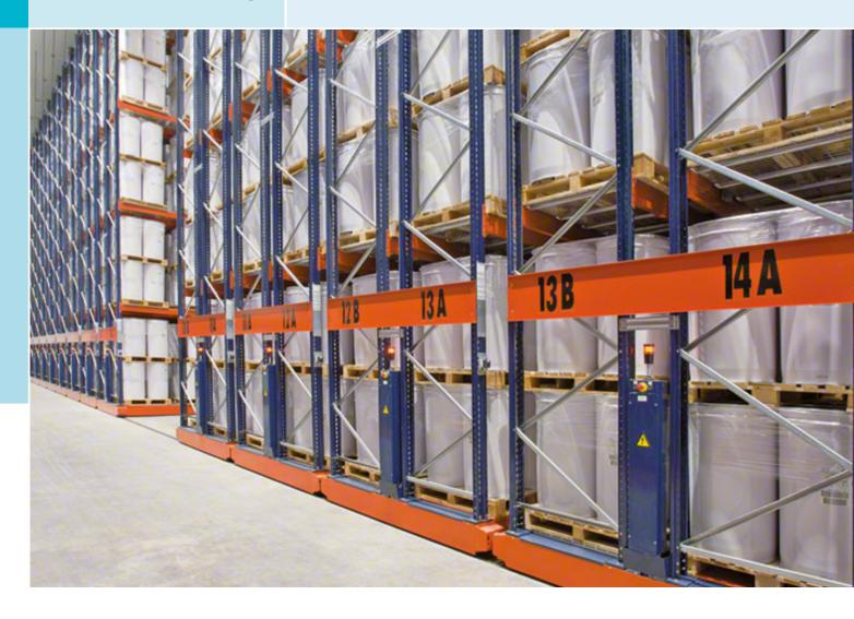
The racking is mounted on mobile bases which move along rails, eliminating the need for multiple access aisles and increasing storage capacity.
