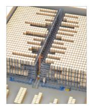
**Automatic Pallet Shuttle** installation with stacker crane The stacker crane carries out movements from the input and output positions in the warehouse to any storage channel. The Pallet Shuttle is tasked with moving the pallets from the cradle of the stacker crane to the location in the corresponding channel. Generally, two high-density storage racking blocks are installed, one on each side of the working aisle.
