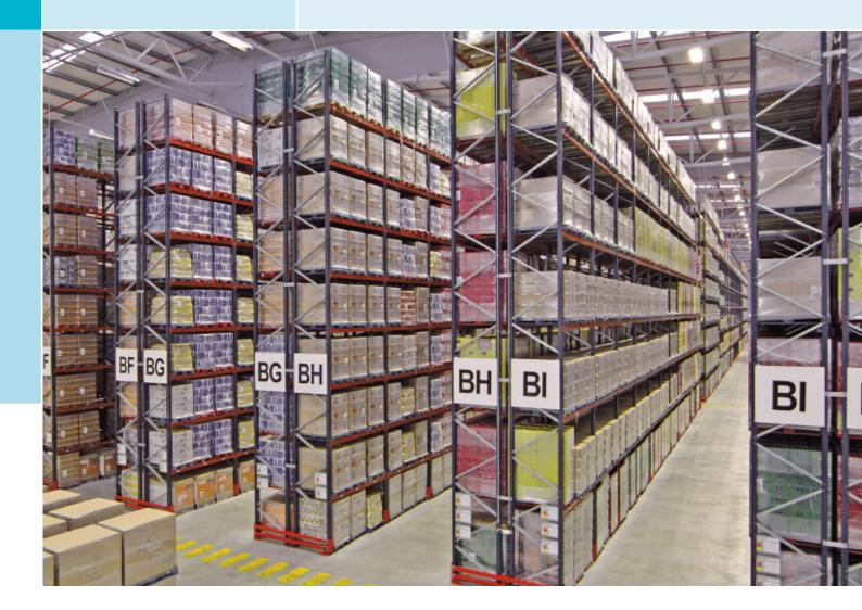
Conventional pallet racking is the best solution for warehouses where it is necessary to store a wide range of articles on pallets.
