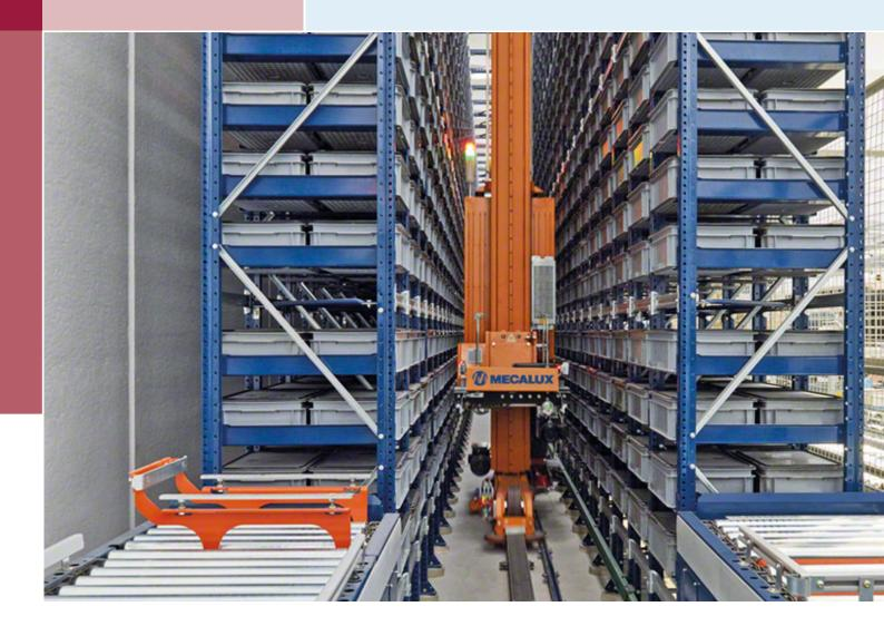
Stacker cranes for boxes are designed to achieve a high level of productivity and manage loads with boxes or trays.
