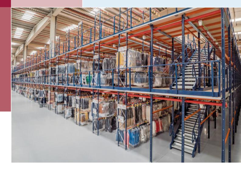
The full use of the warehouse's height is enabled, installing high racks with one or more gangway levels supported by the racks themselves.
