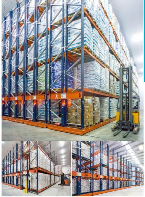
The system includes various safety features, With only one aisle needed for access, using such as aisle optical safety barriers, proximity photocells, reset buttons, etc.
