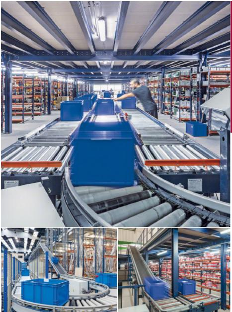
A wide variety of circuits can be configured, with straight sections, curves, inclines and even different levels.
