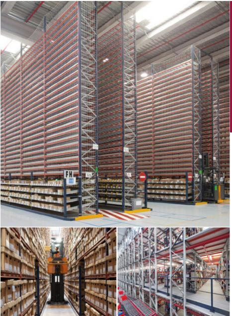
With narrow aisle handling equipment, shelves can reach up to 20 m high.
