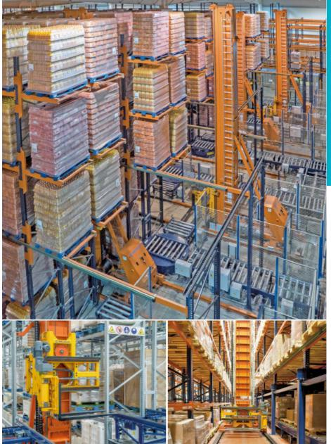
Integrated, trilateral extraction system with a rotating head that picks up and drops off pallets in three positions.
