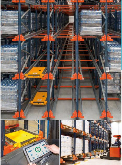
User friendly: the control system uses a tablet with a wifi connection.
