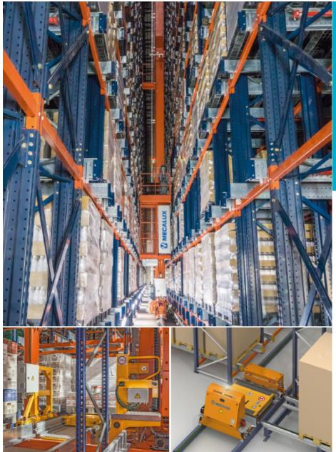
In combination with stacker cranes or pallet lifts, the Pallet Shuttle system reaches a storage height of up to 40 m.
